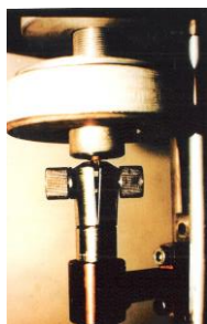
Fig. 3 Testing machine: elastic nut-type head for tractions
