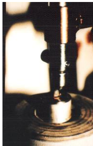
Fig. 2 Testing machine: conical head for oblique compressions
